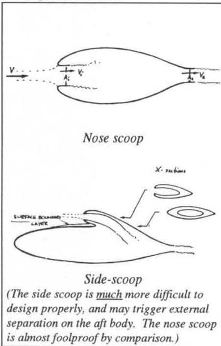
If a scoop is placed near the rider's head, it should have a curled-in leading edge to allow for the deceleration of the flow stream-tube before it gets to the scoop, as shown in the sketch. The scoop must also be offset from the fairing surface so as not to ingest the fairing's boundary layer. This would stall the inside of the scoop duct and prevent maximum deceleration of the incoming air.
