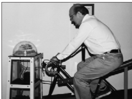
4) Tom Caskey, designer/builder of the "Feet On!" exhibit, pedals the exhibit that shot a spark across a gap inside a vacuum. The long banana seat enabled the exhibit to accommodate various-sized riders.
